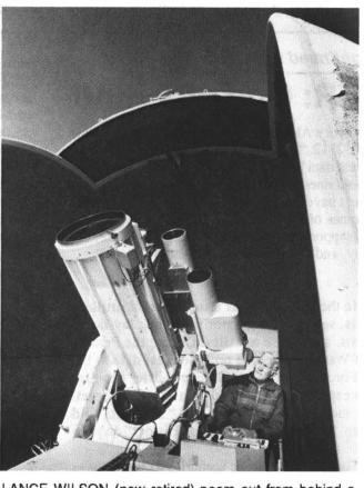
LANCE WILSON (now retired) peers out from behind a tracking telescope housed under a rotating dome.
